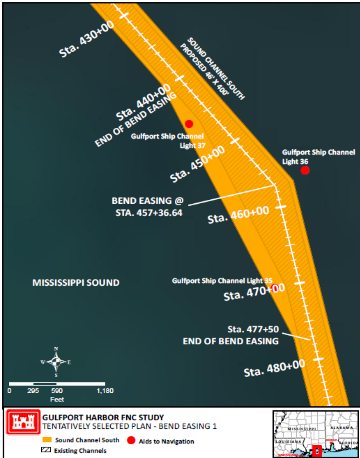
Figure 6-5: Bend 1 - Bend Easing for Sound Channel South
